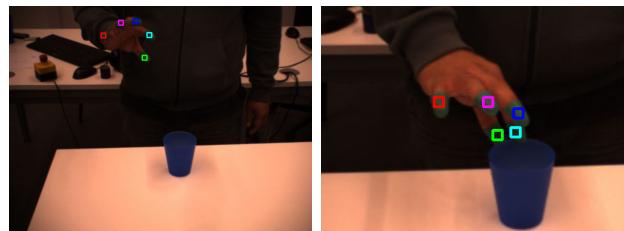
Fig. 4. Left camera views of the tracking method. Red denotes thumb region, light blue the index, blue the middle, pink the ring finger, and red pinkie region
