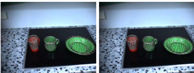
Fig. 3. Effect of the orientation correction on an example scene. Left: no correction. Right: with orientation correction.
