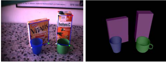
Fig. 7. Recognition and localization result for an exemplary scene. (a) Left input image. (b) 3D visualization of the result.
