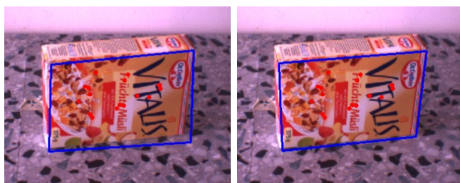
Fig. 5. Difference between 2D localization using an affine transformation only (left) and a homography in the final iteration (right).
