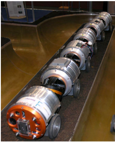
Fig. 7. Snake-like sewer inspection robot MakroPlus
