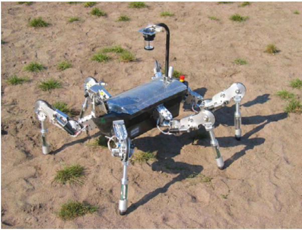
Fig. 6. Six-legged walking machine LAURON IV
