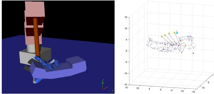
**Fig. 2** Tactile exploration of a phone receiver (left) and acquired 3D point set (right).
